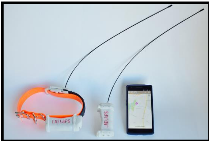
The Laelaps® system – collar, transmitter, and smart phone. Compact and simple.
