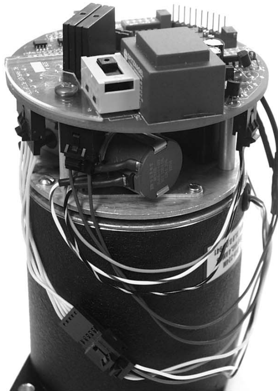
C. ASSEMBLED. NOTE MOTOR ADAPTER JUMPER AND ORIENTATION OF BOARD RELATIVE TO POTENTIOMETER.
