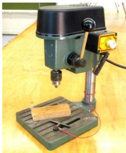
Because these machines are only a foot high, they're limited as to the size of workpieces that can fit into the machine and the size of the drill bits you can use. But I've had no problems with drill bits up to about 3/16" (4.5mm), even drilling steel.
