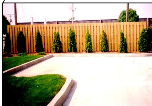
Proposed 8 ft. staggered board wood fence
