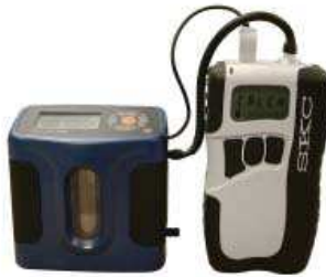
Multiple-point calibration train with CalChek; do not place sample medium in train.
