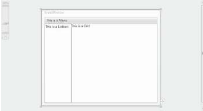
FIGURE 1-6 A DockPanel control that contains a menu, a list box, and a grid.
