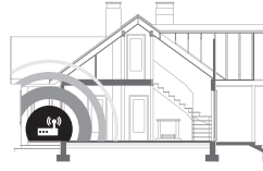
Unsuitable router position
