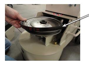
Remove the belt from the motor and driven shaft sheaves as shown in the photo on the left.
