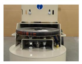
Reverse the previous step to install new belt. Slide motor mount towards the rear of the machine and adjust belt tension, tighten all four (4) bolts as explained above. Replace hood and tighten bolts.
