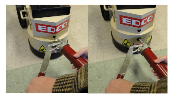
To grease the flange bearings attach the grease gun to the grease fittings as shown in the above photos and give only two (2) pumps on the grease gun weekly. If excessive over lubrication is done grease will leak onto the work surface causing possible damage and wasted cleanup time.
