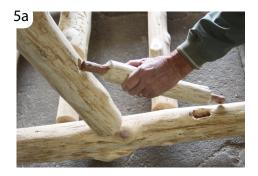
After dry-fitting the pieces, disassemble. Apply a line of Exterior Grade Construction Adhesive halfway in each hole along the sides of each hole. Repeat steps 2-5.
