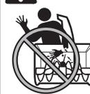
Contact with moving parts inside chute will cause serious injury or death. Shut off engine before unclogging discharge chute. Use clean-out tool, not hands!
