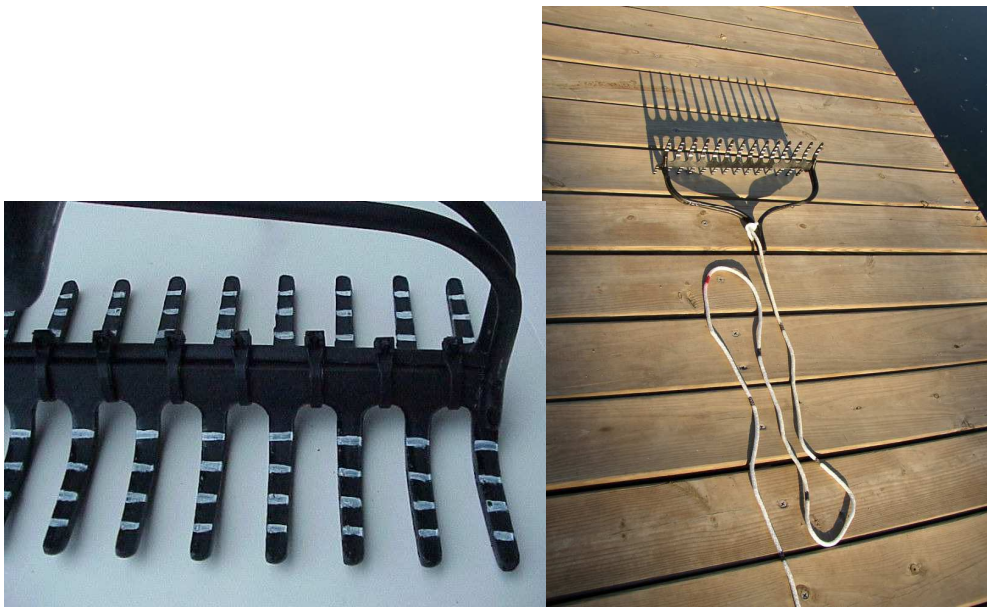
Figure 1: Double-headed rake for aquatic vegetation sampling
