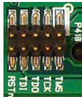
Figure 19 – 10-pin ARM Cortex Debug header (P410)
