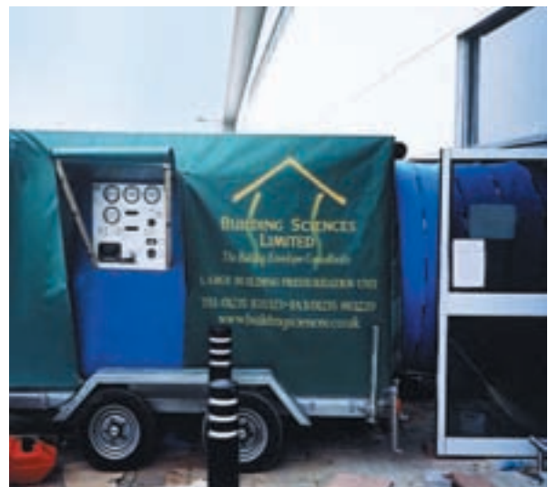
Air pressure testing.
