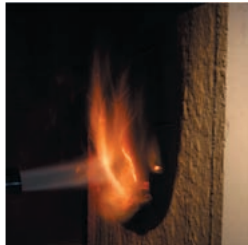
Propane flame test on Kingspan FIREsafe ™ PIR insulation core, after 3 hours.
