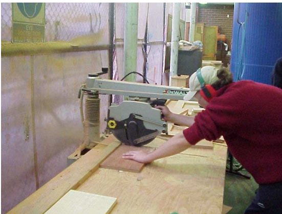
circular saw for rebate joint
