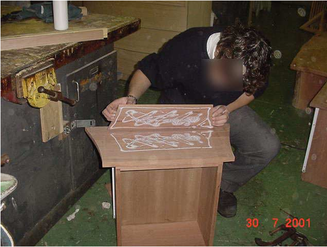
gluing face on
