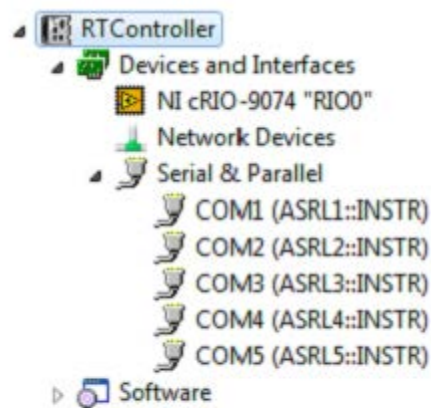
Figure 8.8. Access Your NI 987x serial ports in MAX by installing Scan Engine support.
