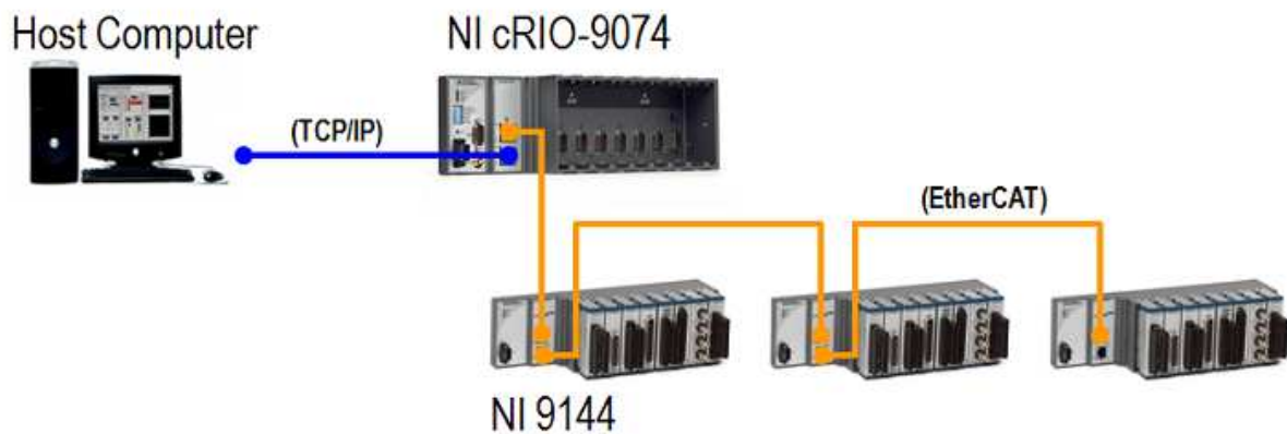
Figure 7.6. The CompactRIO hardware architecture expands time-critical systems using the NI 9144 deterministic Ethernet chassis.
