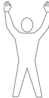
Arms above head in vertical position with palms facing inward. THIS MARSHALLER
