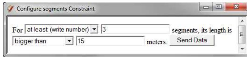
Screenshot 47: Constraint: at least three segments of the current shape measure more than 15 meters
