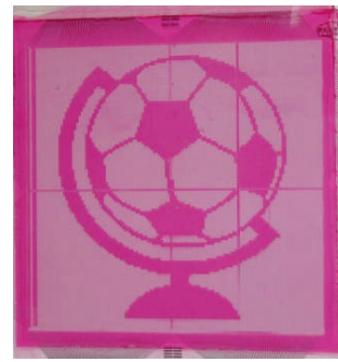
Figure 4. Integrated flexible frontplane with transparent oxide TFT backplane showing pixilation (16384 pixels).
