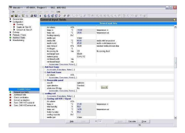
After you have the design of the air handling unit by means of "Lock" button closed, you get above mask for giving all data in principle and necessary of the contained components. You get just suggestions/filled out fields, which you can amend at any time. The number of fields, which you have available, varies depending upon product and software setting by your program distributor.
