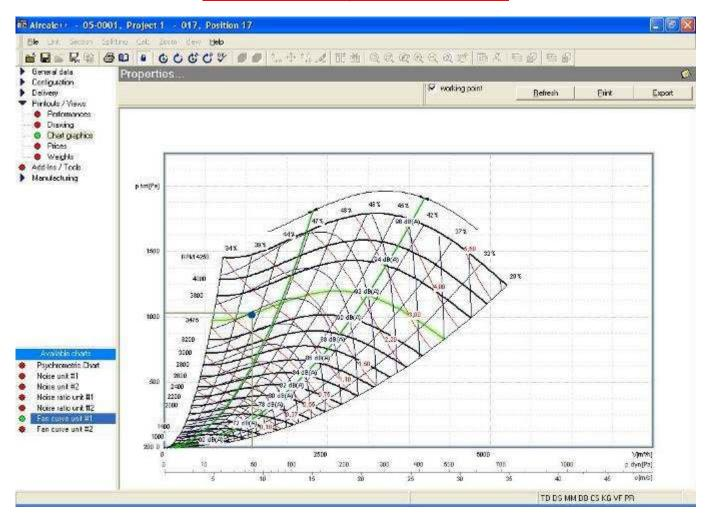
This diagramm shows the fan curve with the working point of the fan. For each unit the programm will create a separate diagramm. (Fan curve unit #1, Fan curve unit #2 in this case)
