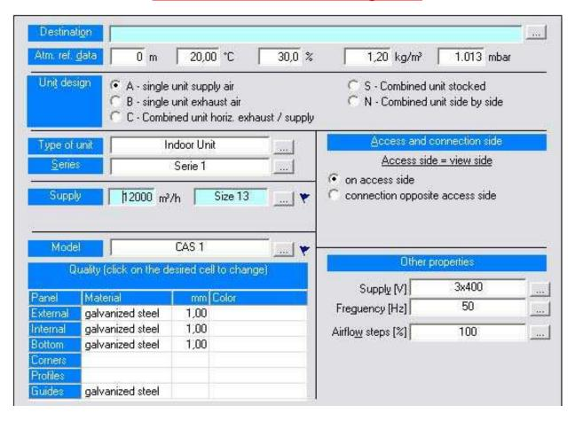
In this mask the user define the unit design, the unit serie, the size, casing and quality, ecc.
