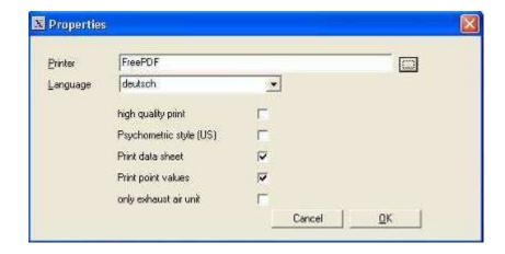
Further: Selection of the printer and the target language, print in a higher resolution, psychometric style (US), printout of the point values, or is to be printed out about only the supply unit on the psychometric chart?
