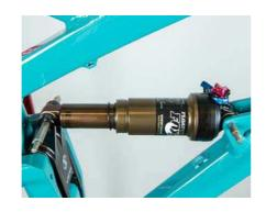
**14.** Install the shock using Fox guide pins to hold it in place.
