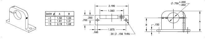
base: universal (\_6\_); pn 160030-\_ (upright mounting; allows 360° rotation about two axes)
