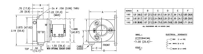
DIMENSIONS: shown with idler cable exit, standard base, and optional sensor cover.
