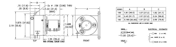
DIMENSIONS: shown with cable guide cable exit, standard base, and optional sensor cover.
