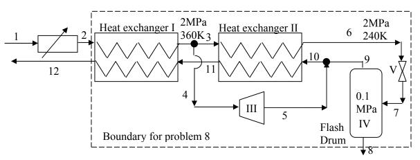
The next few problems consider the liquefaction cycle shown above. The expander is adiabatic and 90% efficient. The flash drum is adiabatic. The operating fluid is refrigerant ethane (chart attached).
