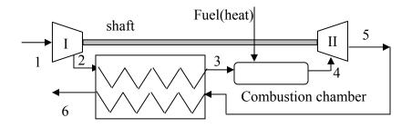
(a) (5) If  $T_1 = 298K$  and the adiabatic compressor is 85% efficient. Find  $T_2$  and <u>W</u>s, I(kW).
