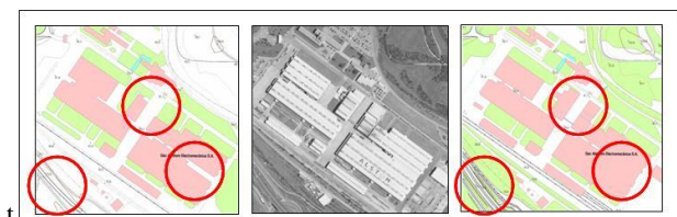
Figure 2. At the left image the original data, at the centre the new image, at the right the updated information. Circles indicate where original information has been partially modified.
