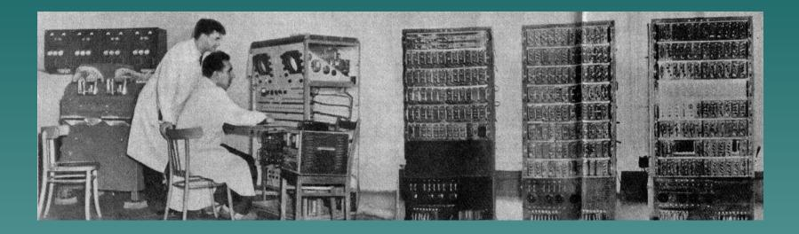
XYZ (L. Łukaszewicz, 1958) – first computer designed and built in Poland. It's electronics included not only tubes, but also on semiconductors (Ge-based diodes).
