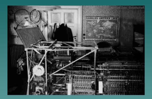
Z1, Z2, Z3 (Konrad Zuse, 1941) – first "generation 0" machines. Z3 was programmed by punched film tape, electromechanical calculator, compatible with Turing concept.
