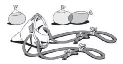
Now use some duct tape to make a cradle inside the funnel. Without this part, when the balloon is released, it will squeeze down inside the hole and burst.
