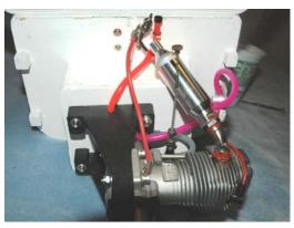
Fuel Filler Valve Installed □
