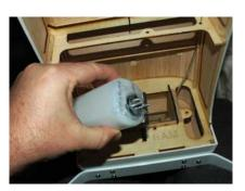
When finished, the tank should be secured; sealed to the firewall, and "floating" on the just slightly compressed foam pad.
