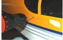
Drill pilot holes, harden with CA and install the canopy.
