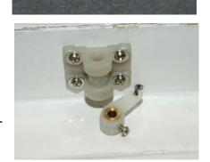
7. Slip the nose gear through the Nose Gear Block and the Steering Arm. Lock down all the set screws.
