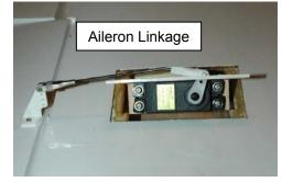
link to flush with the keeper. With the first link as a guide, bend a "mirror image" link for the opposite Aileron. Install and adjust the aileron to neutral. Check for freedom of motion: it may be necessary to widen or lengthen the slot in the servo cover to ASSURE unbinding movement.
