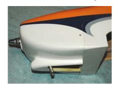
10. THIS STEP IS FOR 2-STROKE ONLY. In order to use the Throttle pushrod
