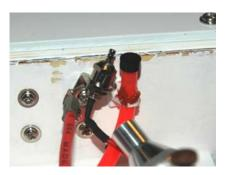
3. Some other pictures for review: an exhaust diverter will be installed but is not shown here so as not to block the view of the remote glow. Also note the overflow tube (capped for flight) and needle valve extension...
