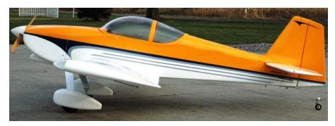
One of the features of this kit is the ability to build it as either a trike or tail dragger, and to switch back and forth if you choose. If you intend from the outset to build yours as a Taildragger than this step will not be necessary. If you removed the covering (Step 7 under "Trike Gear") then use the supplied landing gear covers to cover over the trike gear landing gear mounts.
