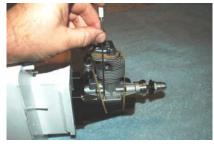
4mm nuts must be used to lock down the engine to the mounts.
