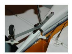
5. The tail wheel control arm is connected to the rudder via two springs. It is important the these be the same length without a lot of stretch. Measure the distance from the bellcrank mounted in step 2 to the steering arm on the bracket. Bend a right angle on one end of both springs, hold them together (forceps work nice) next to the bend, measure back to where the other bend should be and bend both springs together.
