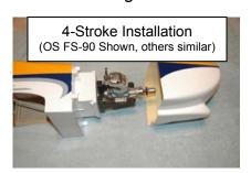
Using a straight edge, check the contouring of the cowl mounting blocks relative to the line of the fuselage. In the picture to the right the block has been sanded and tapered to match the fuselage. Check/correct all six mounting blocks. IF you have to sand the surface then re-seal the wood afterwards with a few drops of thin CA.
