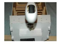
The Main Gear mounts are located under the covering just aft of the lower wing fairing. Cut away the covering to expose the mounts, and seal the edges of the covering.
