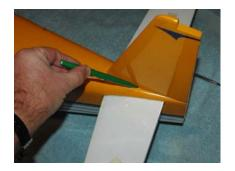
4. Use the small soldering iron to burn & seat the covering along the marker lines, remove the covering from the center of the stabilizer and from the fuselage under the base of the fin.
