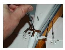
Tail wheel Bellcrank Installed □
