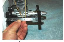
3. For this example, the cowl length was measured as  $5^{1}/_{8}$ " (130.2 mm) so the target dimension: firewall to drive washer is  $5^{3}/_{16}$ " (131.7 mm)
