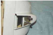
Reinstall the muffler, slip the cowl into place and start filing, sanding, or grinding the cowl
