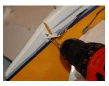
backing plate. When snug, clip off the excess bolt length and file off the burr.
