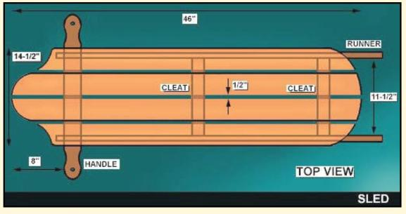
runners and into the cleats and down through the handle. Finish your sled by attaching the slats to the frame made
