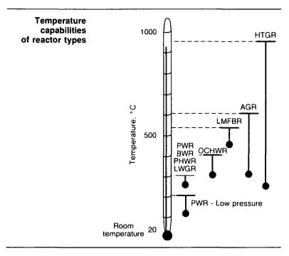
are decisive: the temperature of the produced heat (of primary coolant); and the pressure of produced steam (in some cases).
