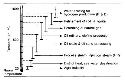
In addition to the maximum temperature of the primary coolant, another important consideration is the temperature difference between coolant inlet and outlet.
