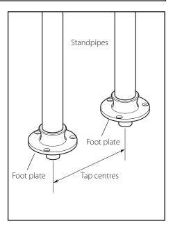
Drill the 3 holes to the required depth and diameter to suit your fixings and floor.
