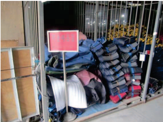
[NON-CONFORMING PRODUCTS IN FABRIC COMPONENTS WAREHOUSE WERE IDENTIFIED AND SEGREGATED]
