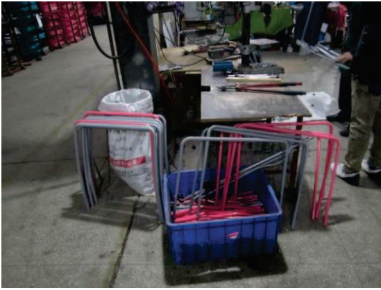
[NON-CONFORMING PRODUCTS WERE NOT IDENTIFIED AND NOT SEGREGATED]
