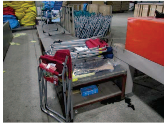
[NON-CONFORMING PRODUCTS WERE NOT IDENTIFIED AND NOT SEGREGATED]
