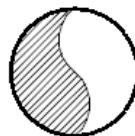
CYLINDER BREAK LINE PARALLEL TO VIEWING PLANE
