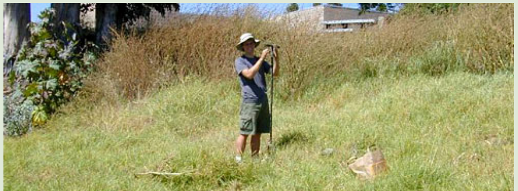
Casey Peters installing index wells to evaluate the hydrology of a potential native wetland.
