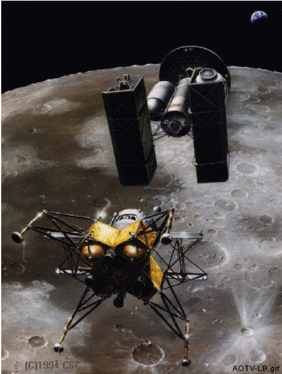
Figure I-3.2.3 The reusable lunar spacecraft fleet, consisting of an AOTV (above) and Lunar Bus (LB, below), artist view by Boeing/NASA
