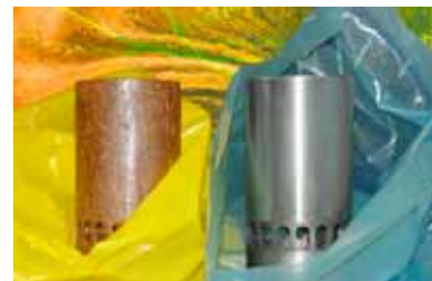
Photo depicts part packaged in plain PE film (left) and part protected with Cortec® VpCI® 126 BIO (right).
