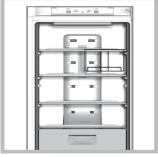
The No Frost system circulates cold air continuously to collect humidity and prevent ice and frost formation. The system maintains an optimal humidity level in the compartment, preserving the original quality of the food, preventing the food from sticking together and making defrosting a thing of the past. Do not block the aeration cells by placing food or containers in direct contact with the refrigerating back panel. Close bottles and wrap food tightly.
