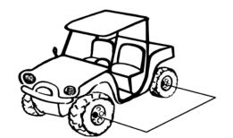
Wheelbase is the distance between the center of the front axle and the center of the farthest rear axle
