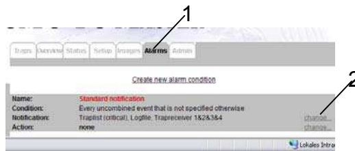
Fig. 45 Configuring alarms for GSM Unit
