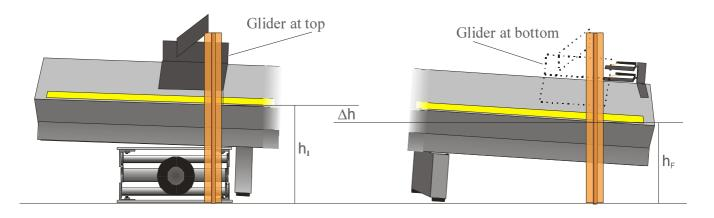
7. Place the glider at the low end of the track so that it just rests against the bumpers and measure the vertical distance from the table-top to the edge of the track at the leading edge of the glider  $(h_f)$ . The change in height ( $\Delta$ h) is given by
