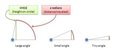
When something moves a tiny amount, such as 0 to 1 degree from our perspective, it's basically going straight up. If you go an even smaller amount, from 0 to .00001 degrees, it's *really* going straight up. The distance traveled (x) is very close to the height (sin(x)).
