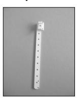
This mounting set sllows to change the height of the swivelling and tilt o + c projection boards, 243..., 244..., 245... und 340..., 341..., 342..., 343..., 344..., 345... und 346... every 5cm up to 30cm. Easy additional mounting possible.
