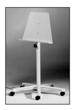
For setting up **o** + **c** boards. 5 legged roller base with stop device on 2 castors. Height adjustable from 78 to 108cm by gas pressure cartridge. Special support for receiving **o** + **c** boards for a mobile and flexible use.
