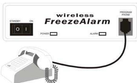
This phone will only be used to program your Wireless FreezeAlarm locally or for locally checking current status of your Wireless FreezeAlarm. It is important to UNPLUG this phone from the front after you are done programming or making any changes.
