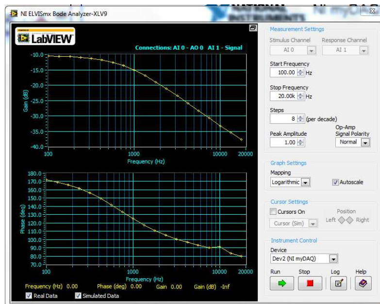
Figure 8: NI myDAQ design lowpass filter Bode Analyzer
