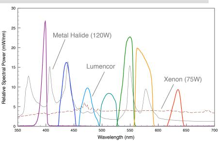
use. Performance exemplified by the light engine outputs in this spectral plot are constant and stable. Unlike traditional lamps, they will not decay significantly with time, or during the course of a multi-day experiment. Researchers and tool designers alike can attain constant, spectrally pure and powerful bands with no need for external filters, filter wheel, shutters, controllers that other light sources require.
