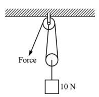
What force must be applied to the rope in the pulley shown in the diagram above to lift the 10-N block?
