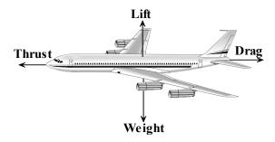
In level flight at constant speed, which pair of forces must be equal?
