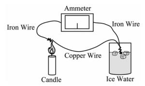
As the temperature difference between the ends of the wires increases, the current in the circuit
