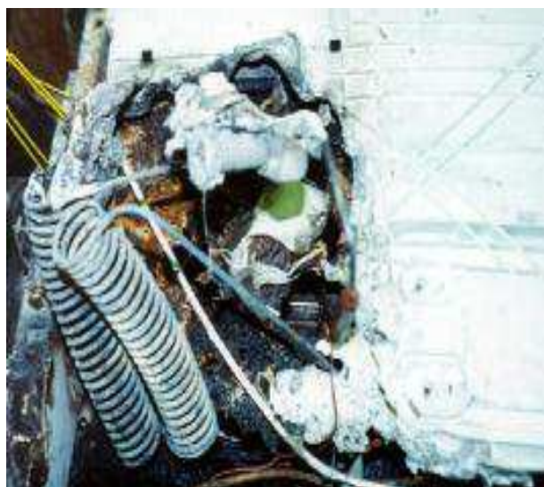
Fridge base showing heat exchanger and fire-damage
