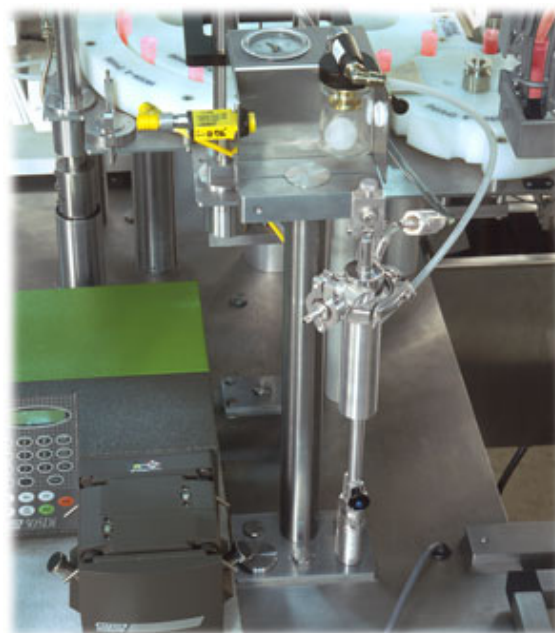
MICROTUBE FILL / FINISH MONOBLOC SIDE VIEW (Shown with DUS with medical grade diaphragm and optional peristaltic fill head.)
