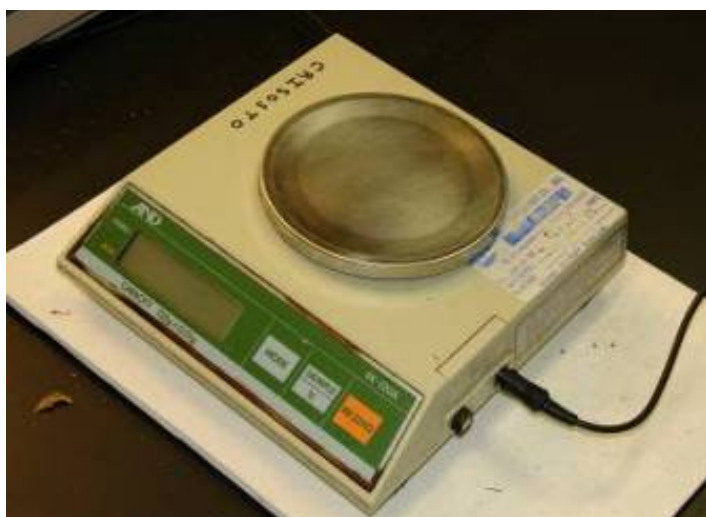
Picture 2. Balance, comparable to Denver Instruments Model MXX-212 with a capacity of 210 g, readability of 0.01 g, taring range of 0-210 g. If purchased from Fisher Scientific includes operations manual and power supply and calibration weight, cat. No. 01-915-02 ($315.40).
