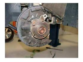
After safely lifting the vehicle to a suitable working height and removing the front wheels start removing the stock brake components. Begin with the calipers and brake lines and then the carrier and rotor. It is a good idea to thoroughly clean and prepare the rotor hub to avoid any debris from causing a misalignment of the new brake components.
