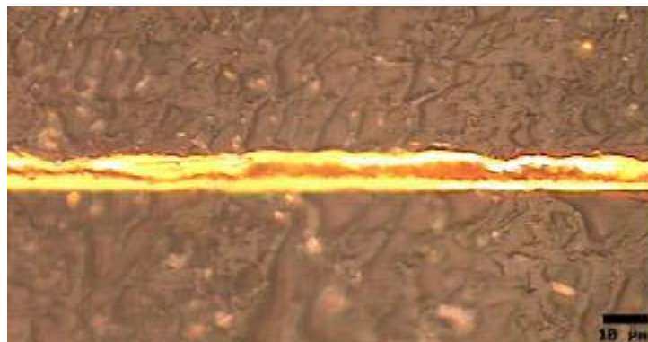
Figure 14. Cross section of coil indicating the electrode thickness to be about 8 µm.
