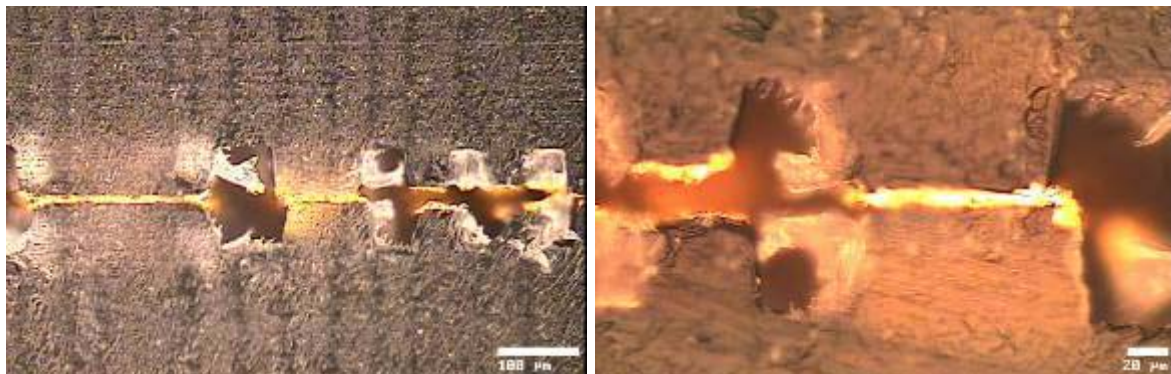
Figure 13. The pictures depict a cross section of a coil. The underpass has not collapsed during assembly, and as can be seen in the right image the size of the underpass is about 20 µm.
