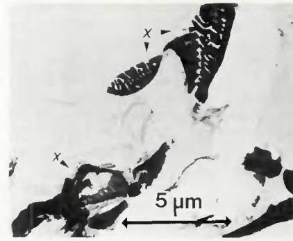
Fig. 16—Extraction replica TEM micrograph from a hot crack in heat 3, 97% Ar-3% N 2 shielding gas, showing eutectic chi phase (arrow) along the crack; primary austenite mode. Note the lamellar appearance of the chi phase
